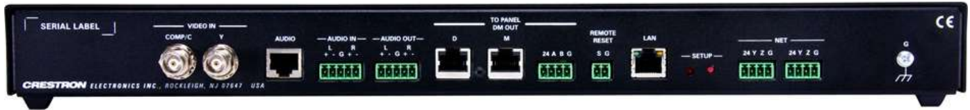
DGE-1 – Rear View
