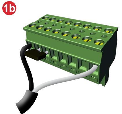
1b 70 V / 100 V operation (keep jumper on 8 \Omega and Jumper positions)
