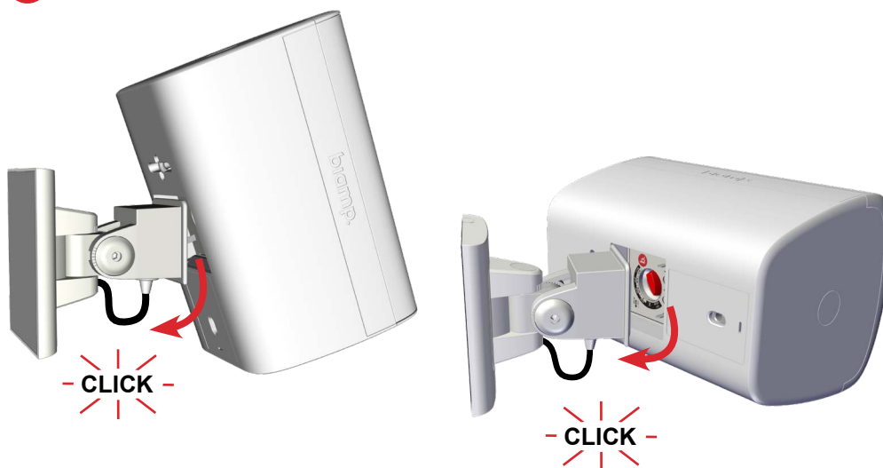
Rotate and press the loudspeakers on the ClickMount bracket
